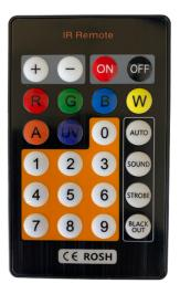
Press **Auto/Sound/Strobe** to switch on or off Auto mode, Sound Active mode and Strobe mode, respectively.
